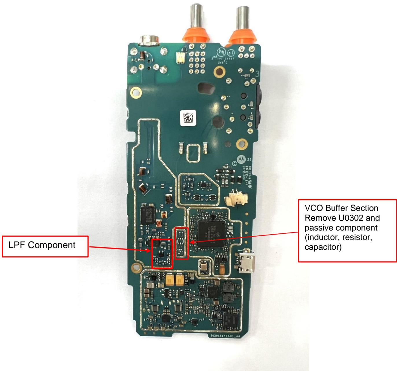
**Exhibits 9C - RF board with Shields (Bottom)**
