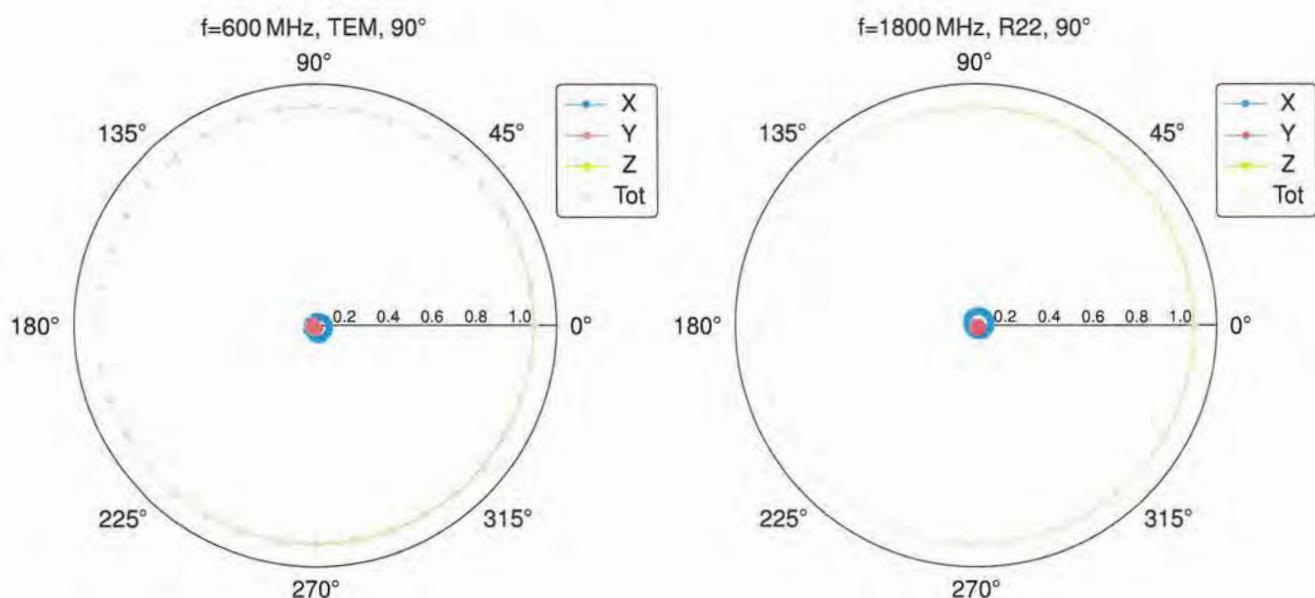
**Receiving Pattern ( $\phi$ ),  $\vartheta = 0^\circ$**
