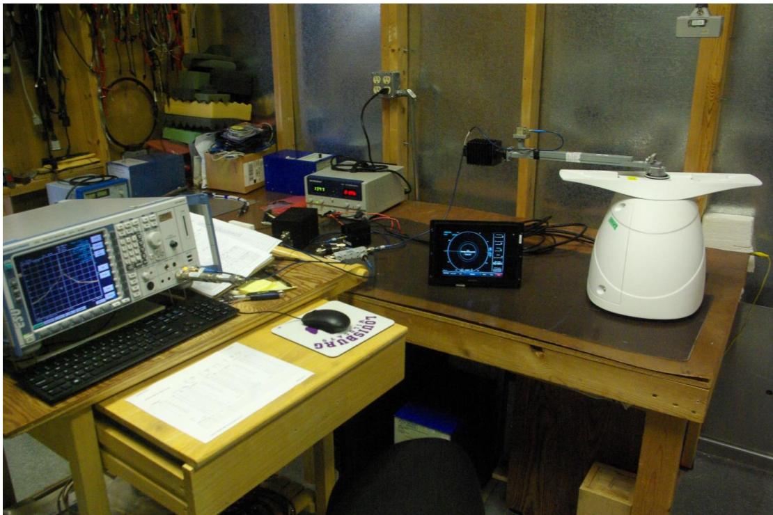
Antenna Port Conducted Emissions Test Setup
