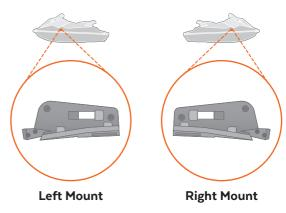
Once, as recommended, the mounts have been installed by a licensed Yamaha dealer, slide the left and right speakers into their respective mounts. When each speaker slides in, the spring-loaded Pin Latch will be pushed out and spring back into place. Do not stop sliding each speaker until the Pin Latch returns to its locked position.
