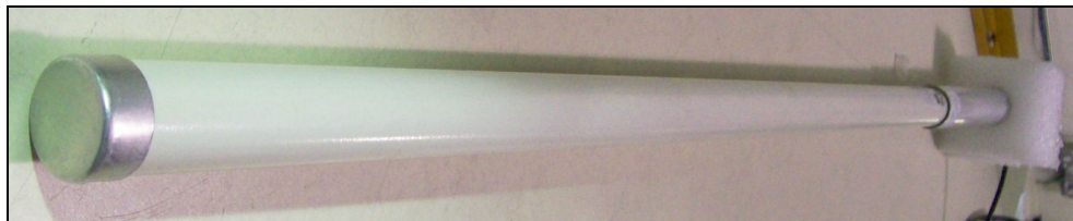
Figure 5: External Photo – Dipole Antenna
