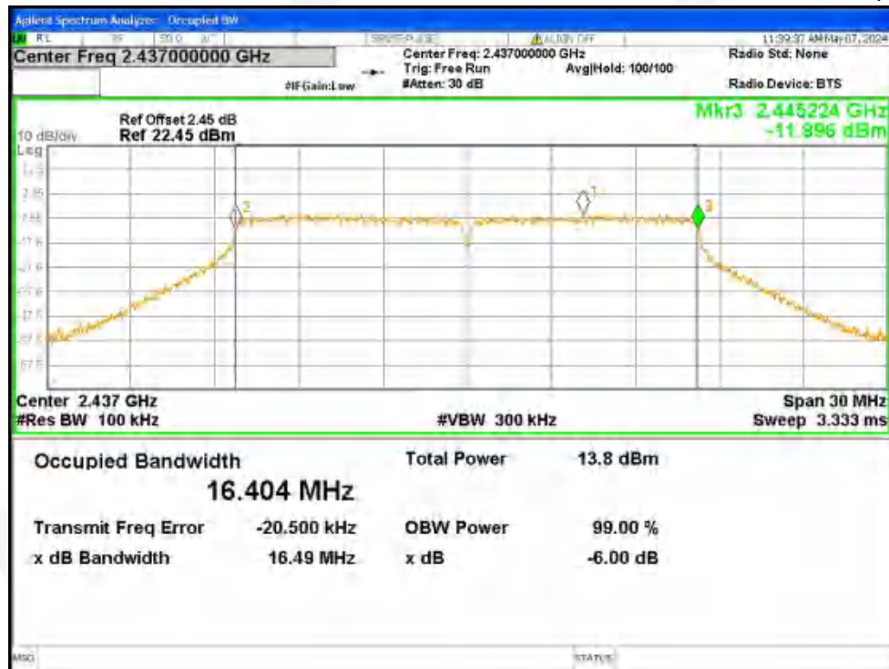
-6dB Bandwidth NVNT g 2437MHz Ant2
