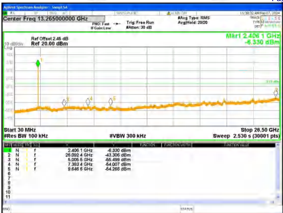
Tx. Spurious NVNT g 2412MHz Ant2 Emission
