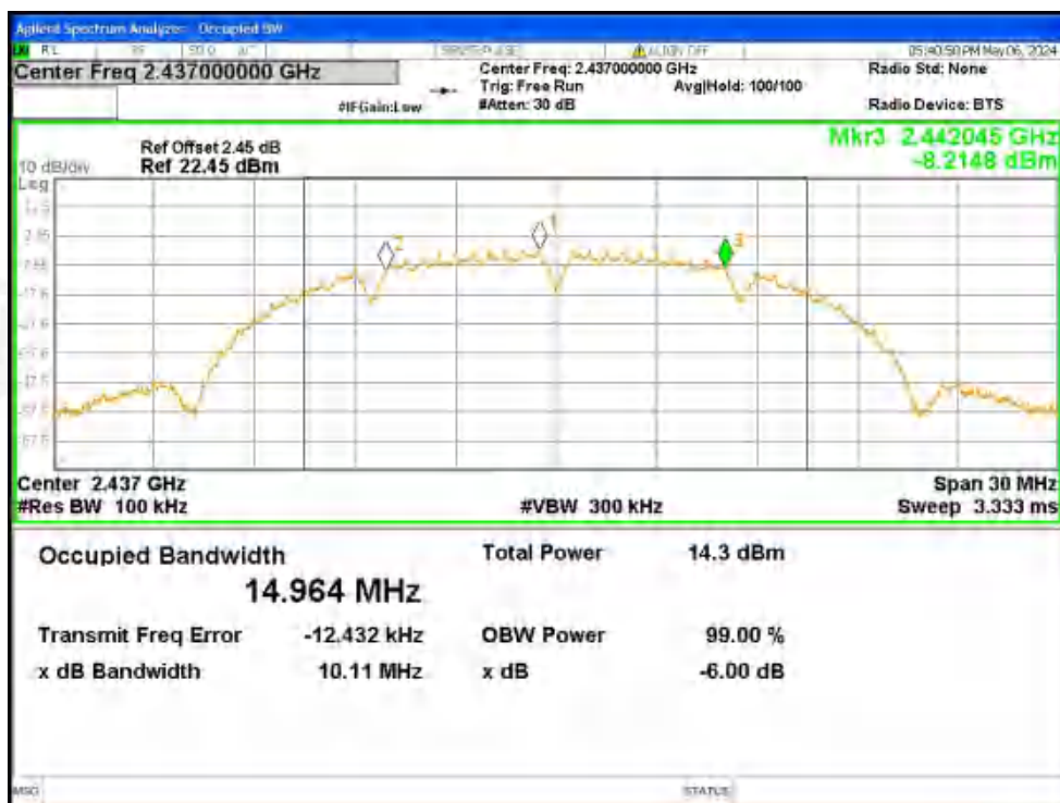
-6dB Bandwidth NVNT b 2437MHz Ant1
