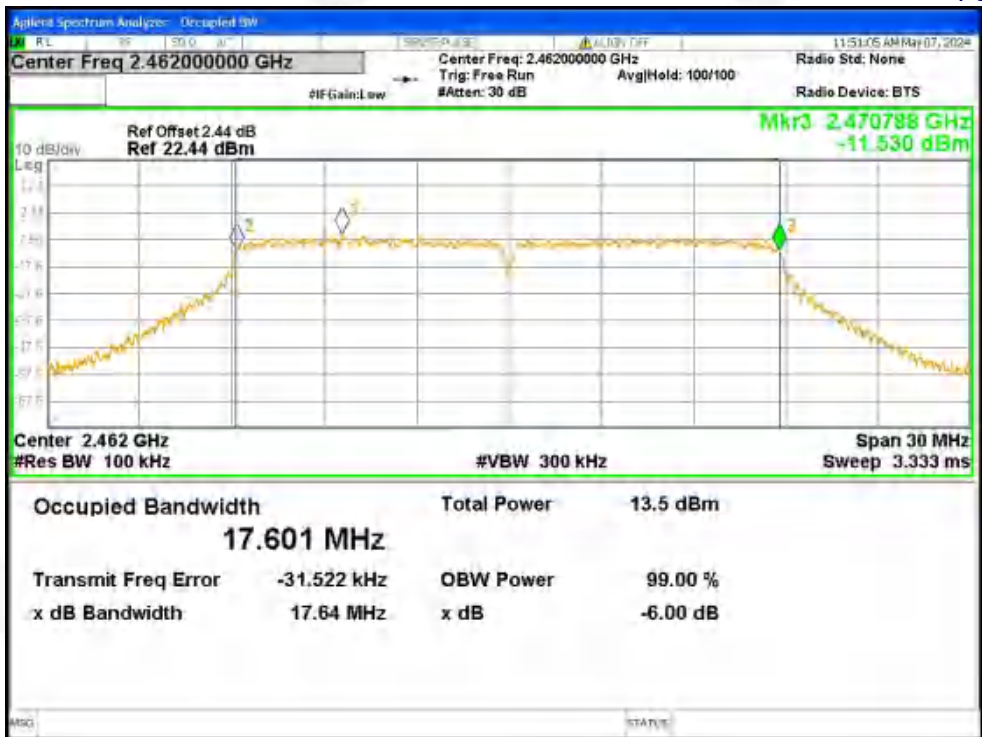
-6dB Bandwidth NVNT n20 2462MHz Ant2
