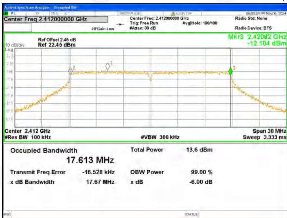
-6dB Bandwidth NVNT n20 2412MHz Ant1
