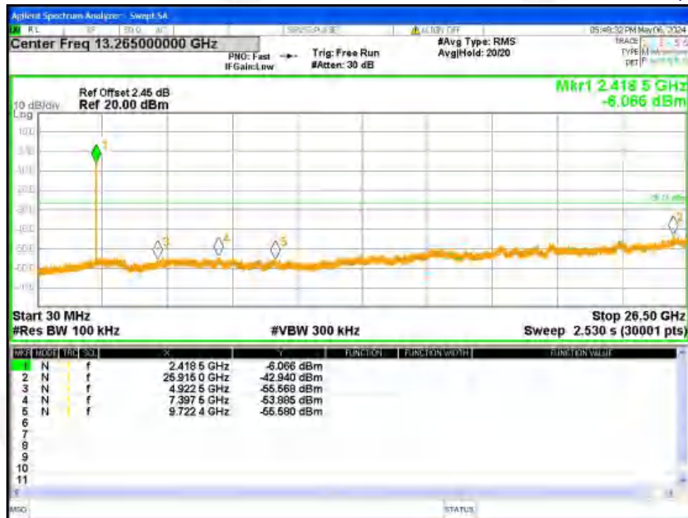
Tx. Spurious NVNT g 2412MHz Ant1 Emission
