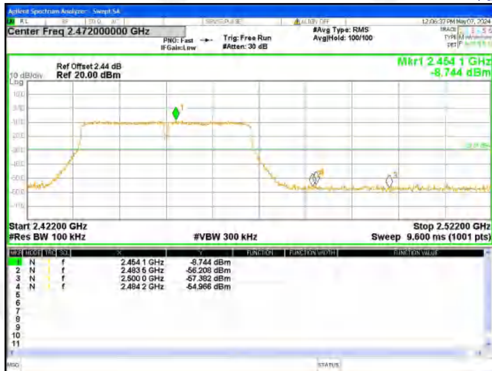
Band Edge NVNT n40 2452MHz Ant2 Emission
