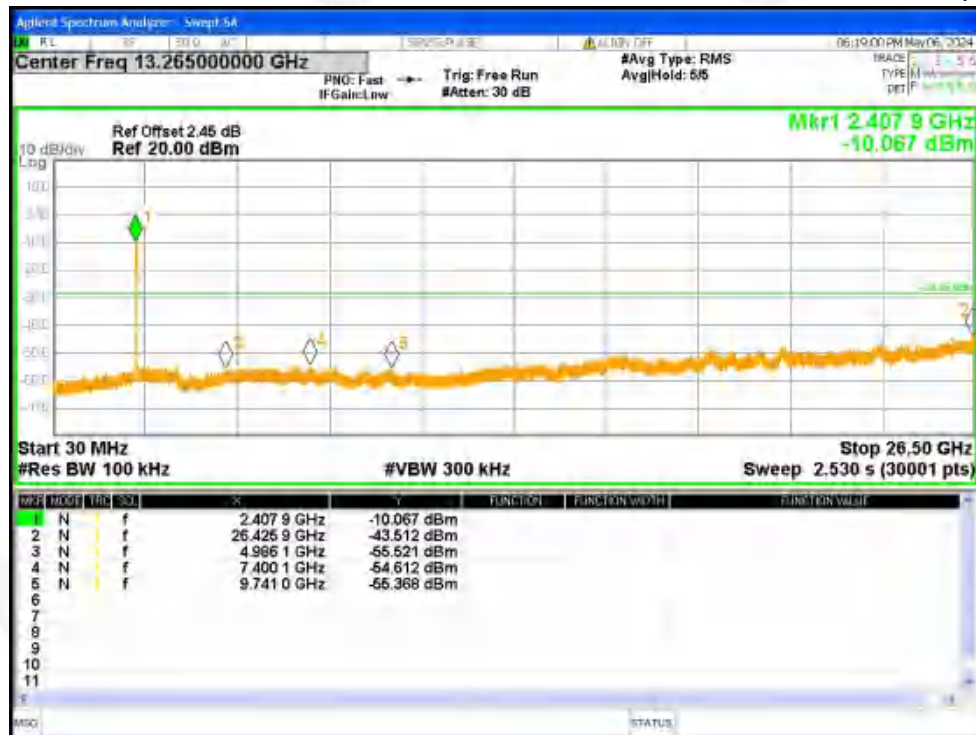
Tx. Spurious NVNT n40 2422MHz Ant1 Emission
