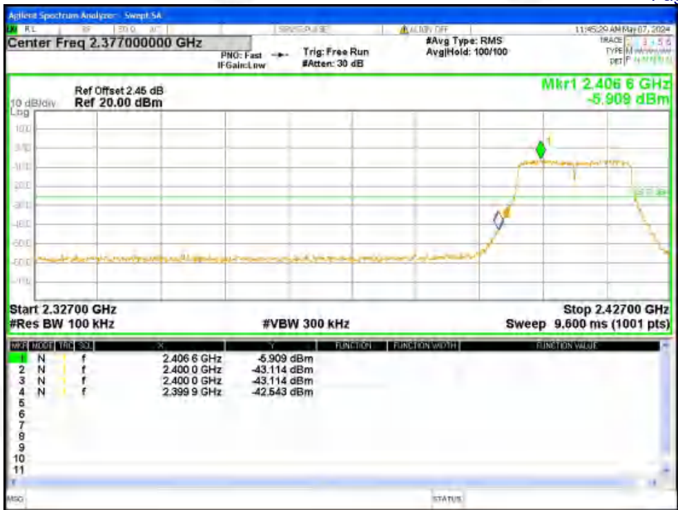
Band Edge NVNT n20 2412MHz Ant2 Emission
