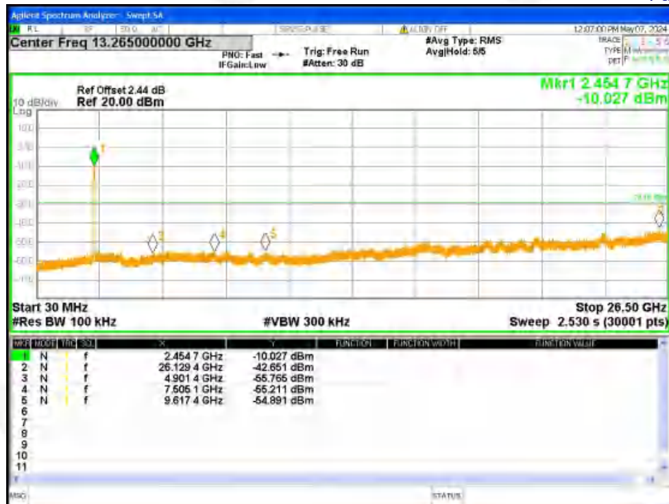
Tx. Spurious NVNT n40 2452MHz Ant2 Emission
