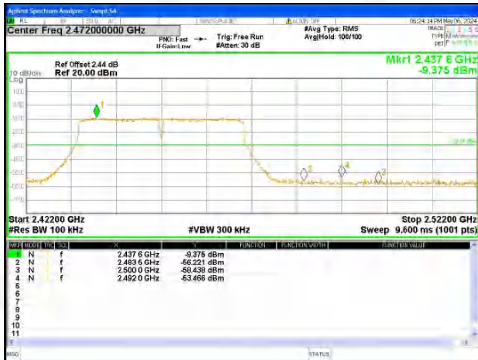
Band Edge NVNT n40 2452MHz Ant1 Emission
