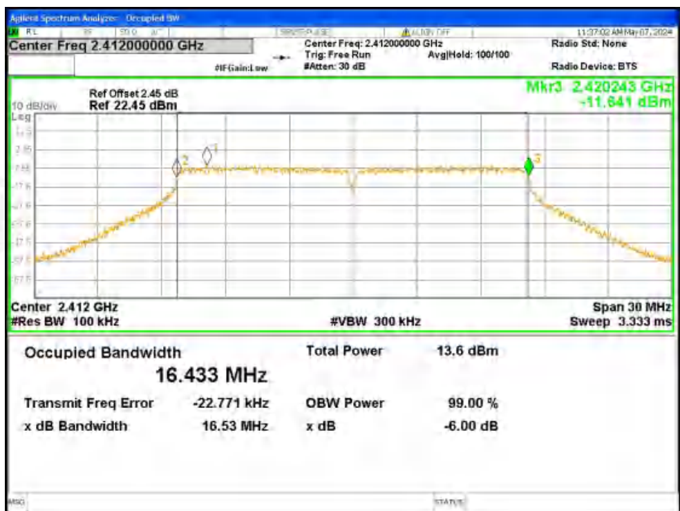
-6dB Bandwidth NVNT g 2412MHz Ant2
