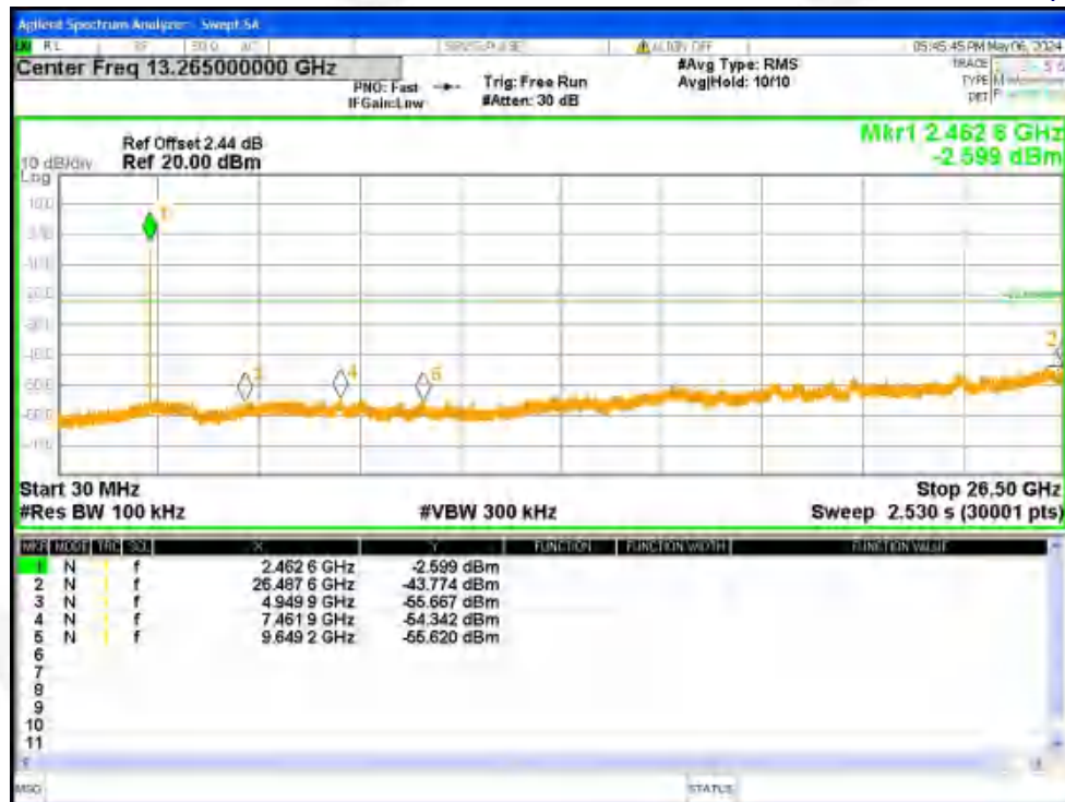
Tx. Spurious NVNT b 2462MHz Ant1 Emission
