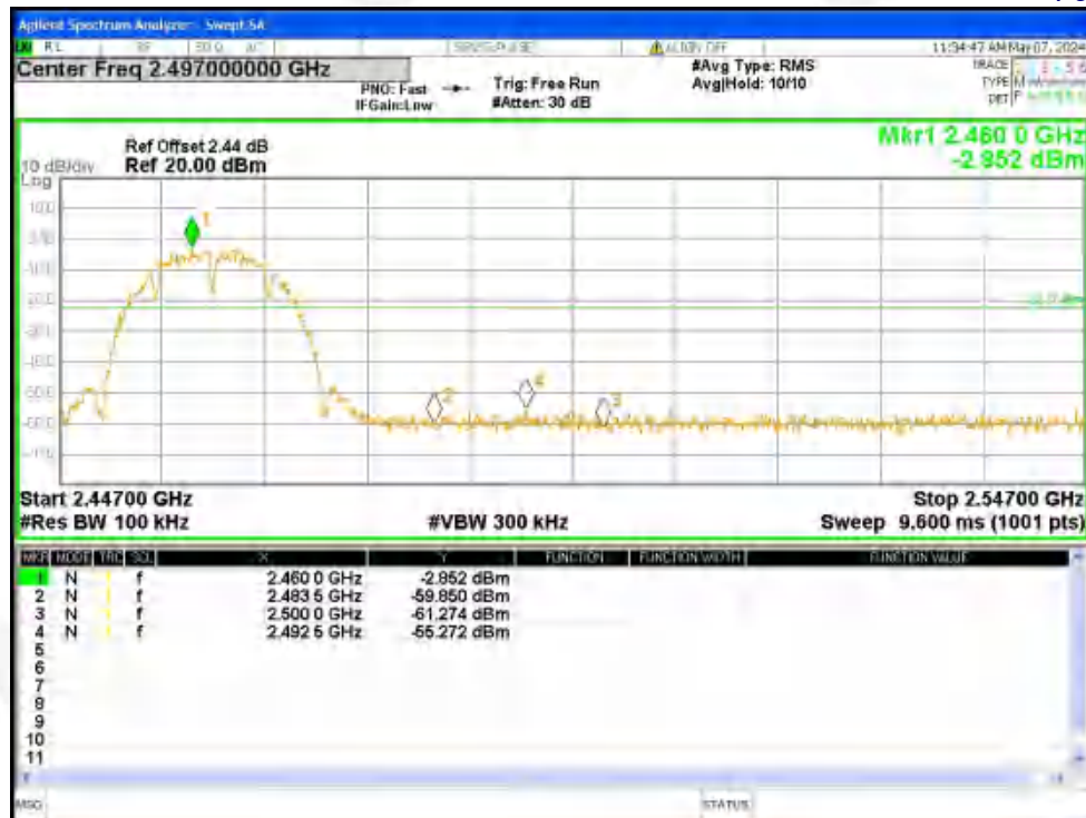
Band Edge NVNT b 2462MHz Ant2 Emission
