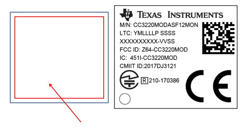
Information is laser etched onto the metal can of the module
