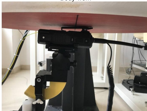
Back side with Speaker Microphone (0mm)
