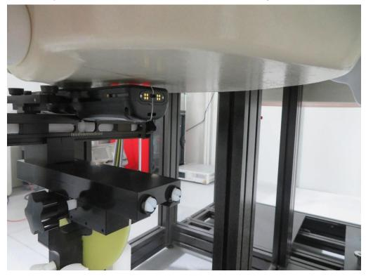
Description: Body Back position for WWAN Antenna with 5mm gap
