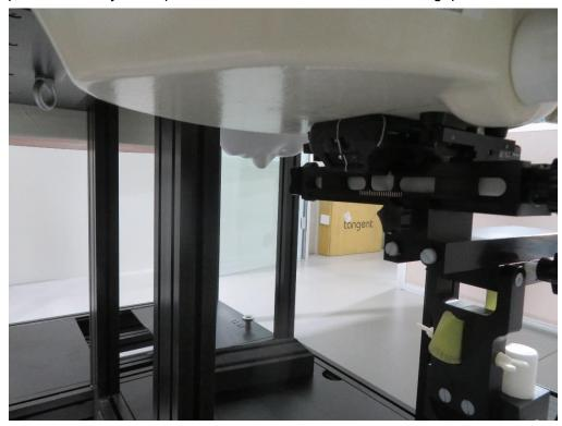
Description: Extremity Back position for WLAN Antenna with 0mm gap
