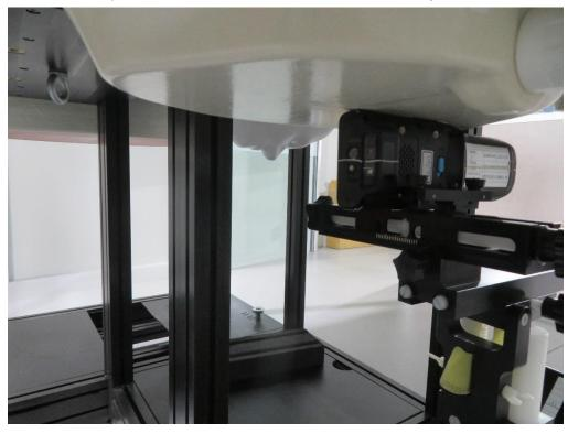
Description: Extremity Right position for WLAN Antenna with 0mm gap
