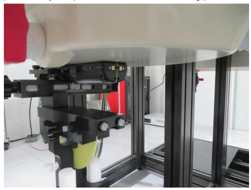
Description: Extremity Back position for WWAN Antenna with 0mm gap
