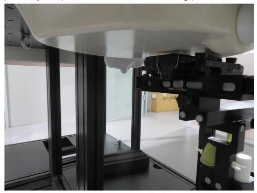
Description: Body Back position for WLAN Antenna with 5mm gap
