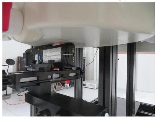
Description: Extremity Right position for WWAN Antenna with 0mm gap
