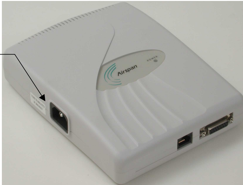
Figure 9-14: Location of SDA-1 power port
