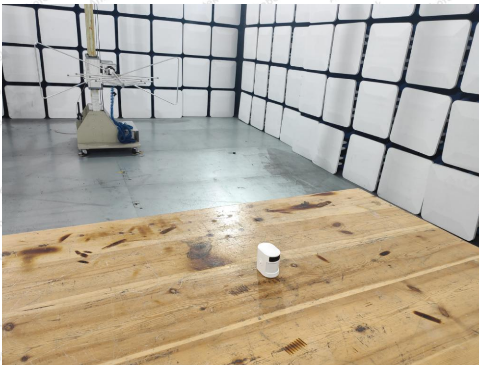
Photo of Radiation Emission Test
