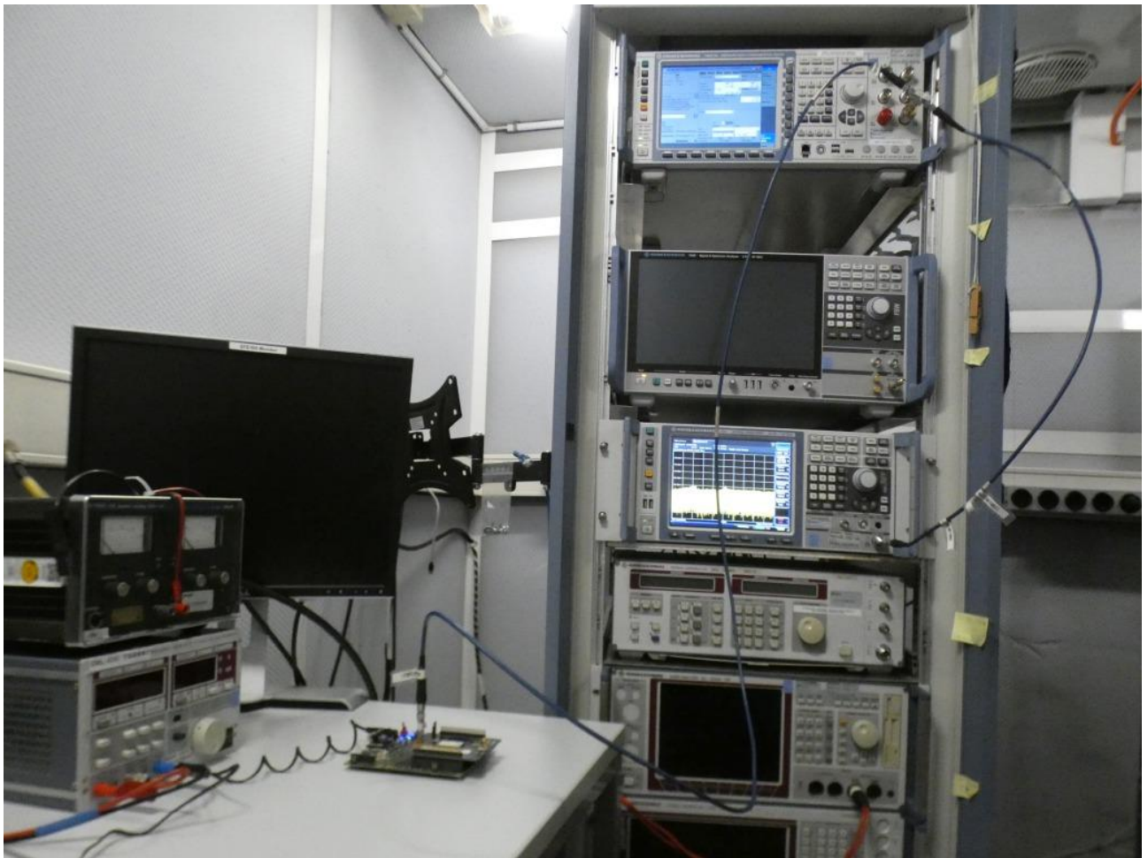
Photo 5: Test setup for conducted measurements (Radio Lab; FCC part 22, 24 and 90, ANSI 63.26)
