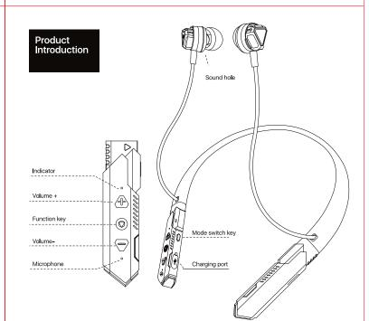
BT pairing: Press and hold the Function key for 5s, and the earphone will turn on and enter the pairing state with a prompt tone "Power On Pairing", and the indicaotr light flashes. Find the pairing name "VC02" on the phone and click to connect with the earphone. (If you can't find the BT pairing name, turn off and then turn on the phone BT to try again.) Connection succeeded: with a prompt tone "Connected".
