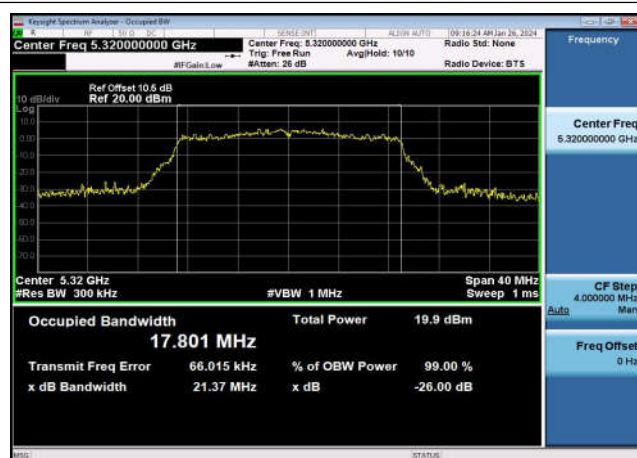
U-NII-2a 99% & 26dB Bandwidth-802.11n(20MHz) ,5320MHz,Ant1
