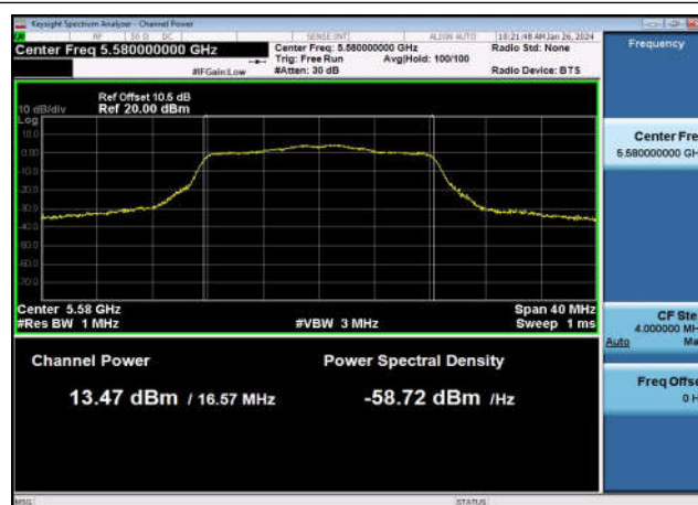
U-NII-2c Output Power-802.11a(20MHz) ,5580MHz,Ant1
