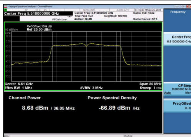
U-NII-2c Output Power-802.11ac(40MHz) ,5510MHz,Ant1
