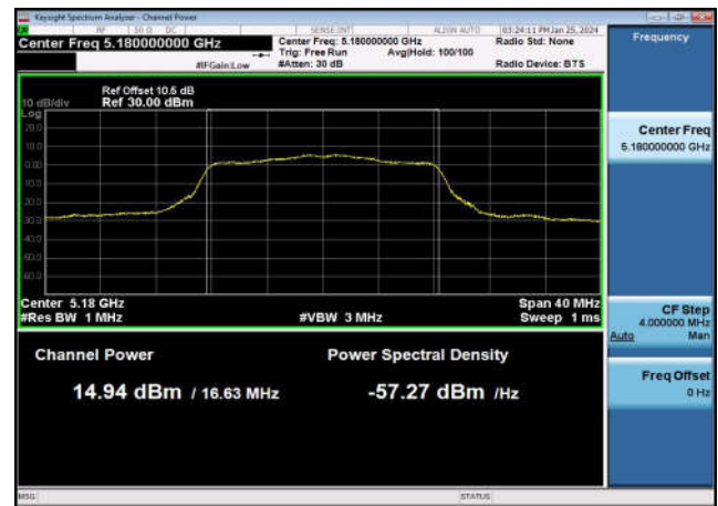
U-NII-1 Output Power-802.11a(20MHz) ,5180MHz,Ant1
