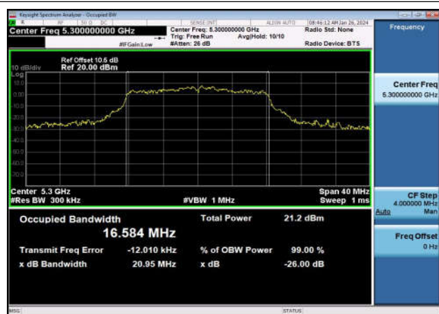
U-NII-2a 99% & 26dB Bandwidth-802.11ac(20MHz) ,5260MHz,Ant1
