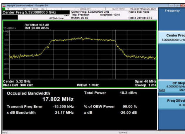
U-NII-2a 99% & 26dB Bandwidth-802.11ac(40MHz),5310MHz,Ant1
