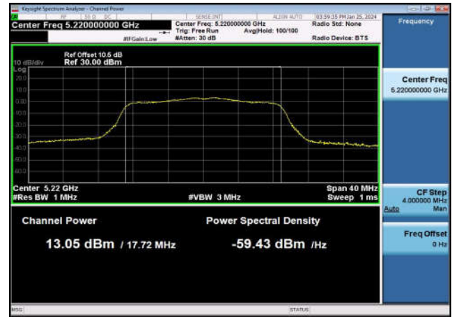
U-NII-1 Output Power-802.11n(40MHz) ,5190MHz,Ant1
