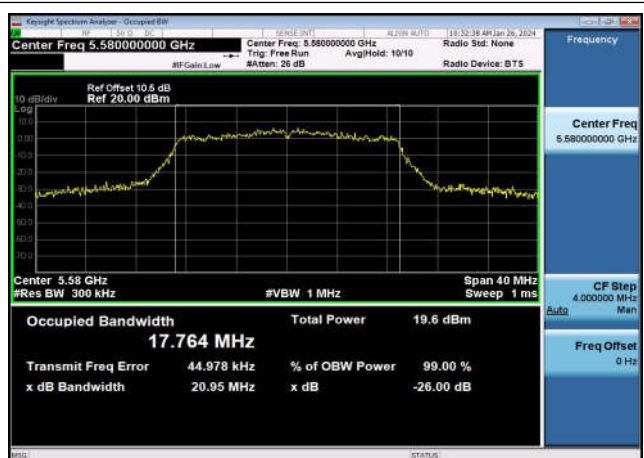
U-NII-2c 99% & 26dB Bandwidth-802.11n(20MHz),5580MHz,Ant1
