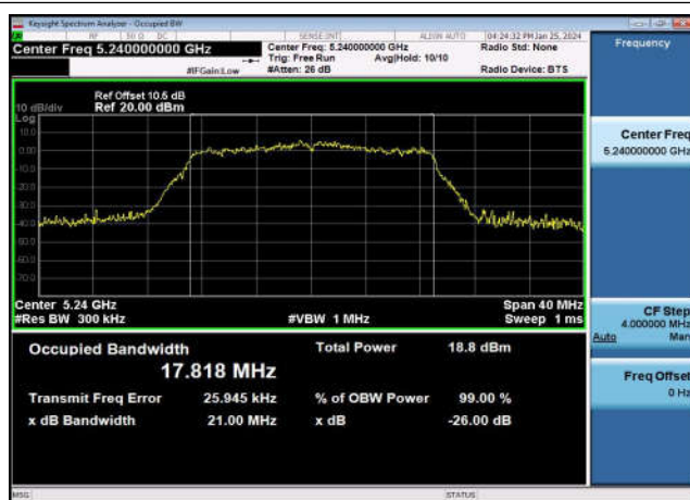
U-NII-1 99% & 26dB Bandwidth-802.11ac(20MHz) ,5240MHz,Ant1
