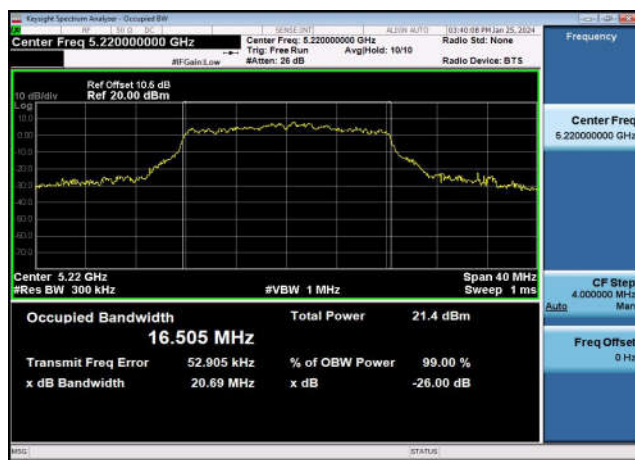
U-NII-1 99% & 26dB Bandwidth-802.11ac(20MHz) ,5180MHz,Ant1
