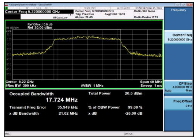
U-NII-1 99% & 26dB Bandwidth-802.11n(40MHz) ,5190MHz,Ant1
