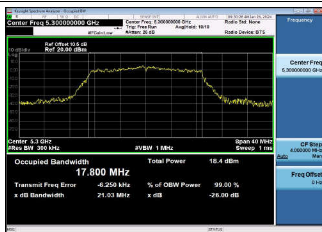
U-NII-2a 99% & 26dB Bandwidth-802.11ac(20MHz) ,5300MHz,Ant1
