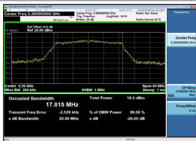
U-NII-2a 99% & 26dB Bandwidth-802.11ac(20MHz) ,5260MHz,Ant1
