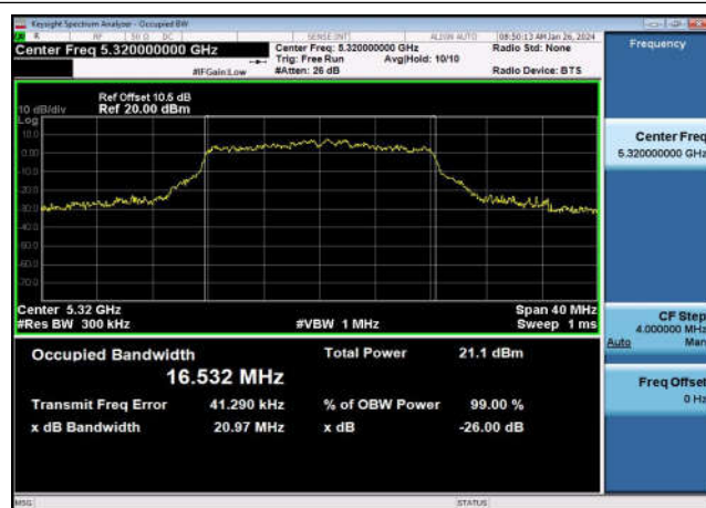
U-NII-2a 99% & 26dB Bandwidth-802.11ac(20MHz) ,5300MHz,Ant1
