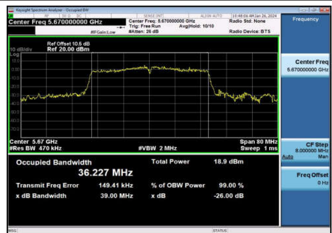
U-NII-2c 99% & 26dB Bandwidth-802.11a(20MHz) ,5580MHz,Ant1
