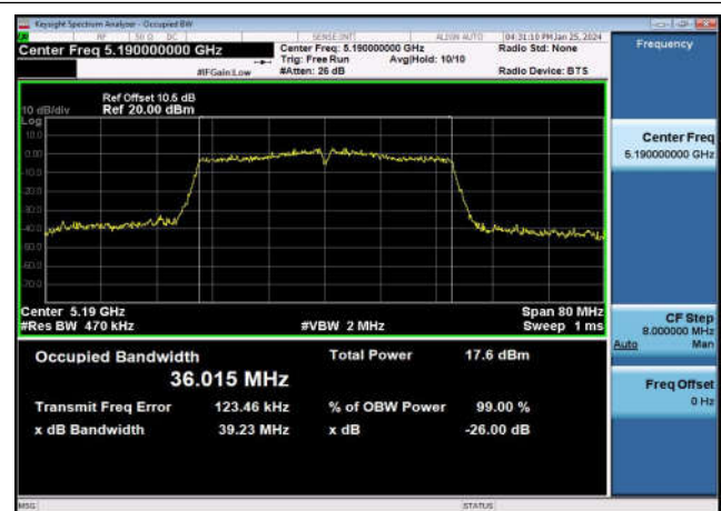
U-NII-1 99% & 26dB Bandwidth-802.11ac(40MHz) ,5190MHz,Ant1
