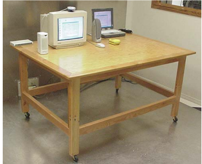
Photograph H-1 – AC Powerline Conducted Emission Configuration
