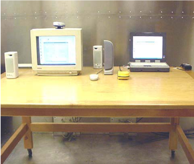
Photograph H-1 – AC Powerline Conducted Emission Configuration
