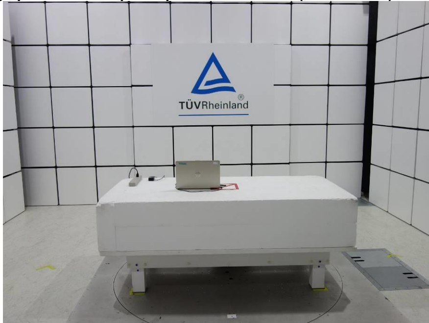
Photograph 2: Test Setup for Spurious Emissions (Front View 2)
