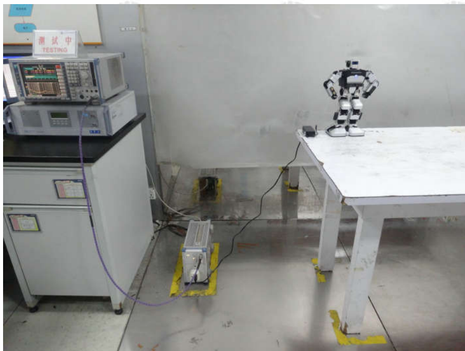
Conducted Emissions Test Setup
