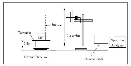
(C) Radiated Emission Test-Up Frequency Above 1GHz
