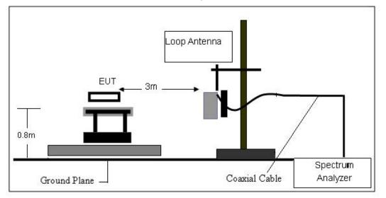
(B) Radiated Emission Test-Up Frequency 30MHz~1GHz
