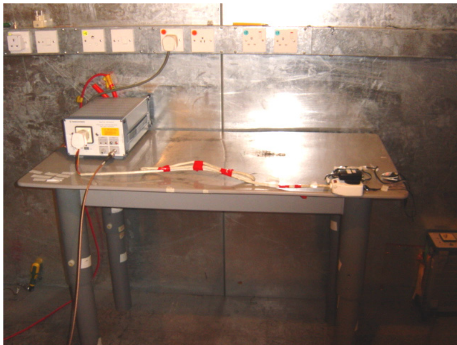
Set-up for Disturbance Voltage on AC Mains
