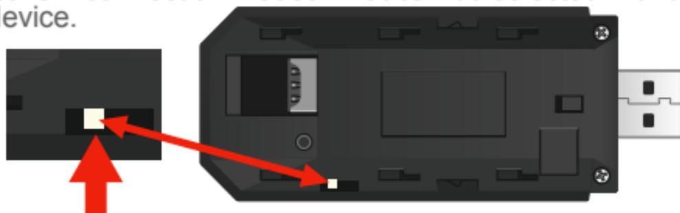
**Right** ➡ : 🌐 LAN NETWORK MODE : In this mode you can install the Windows drivers. The device will show up as a LAN connection.
