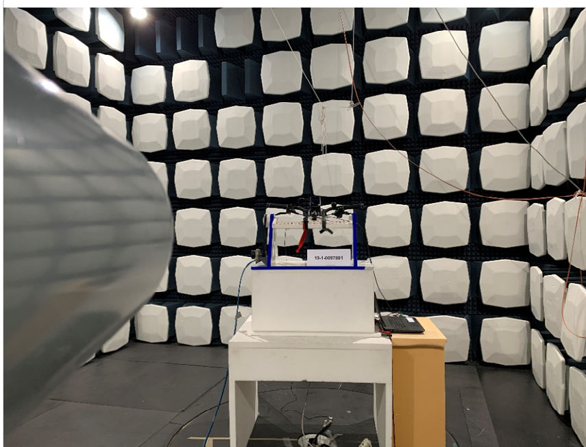
Photograph 4: EUT Setup in the fully anechoic chamber, overview
