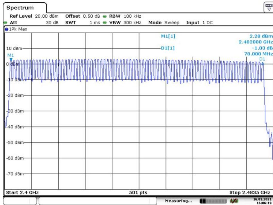
**EDR Mode ( $\pi/4$ -DQPSK)**
