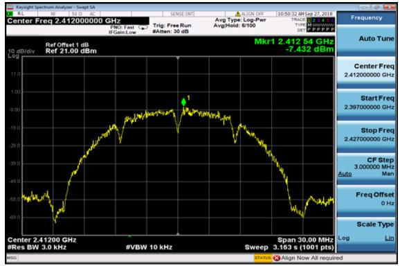
**Power Spectral Density Test Plot (CH-Mid)**
