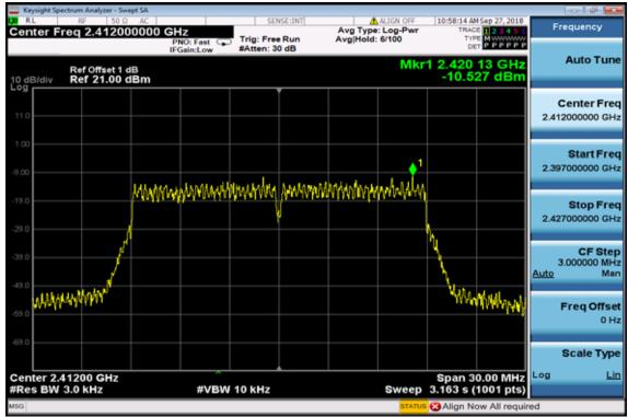
Power Spectral Density Test Plot (CH-Mid)
