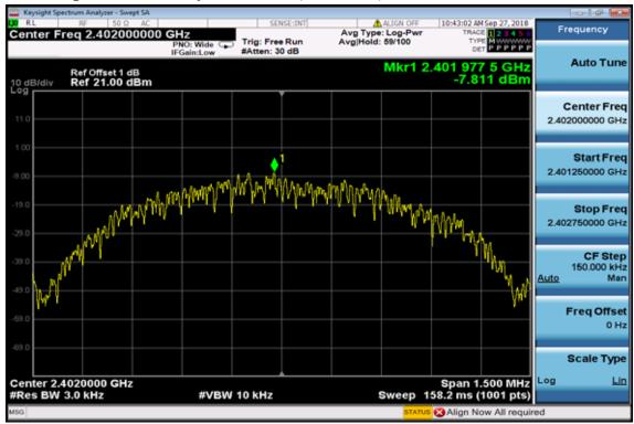
**Power Spectral Density Test Plot (CH-Mid)**
