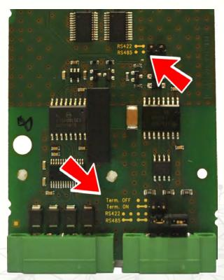
Figure 49: Connection of jumpers
