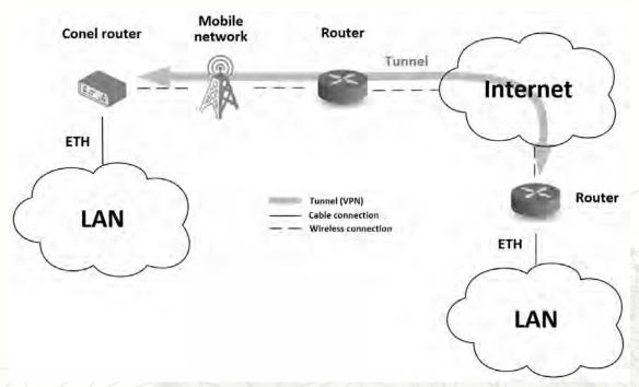
Figure 3: Using VPN tunnel
