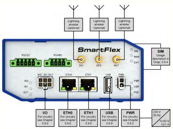
Figure 55: Router connection
