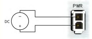
Figure 30: Connection of power supply
