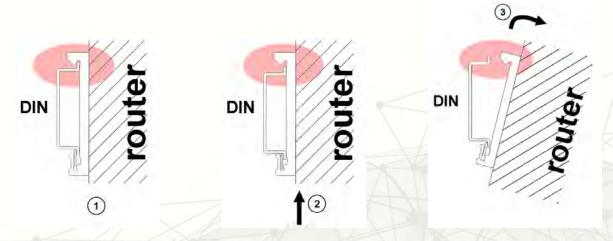
Figure 27: Removing from the DIN rail
