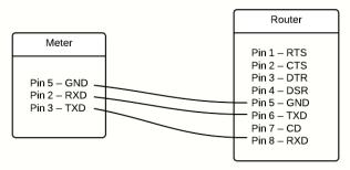
Figure 45: Meter connection to router
