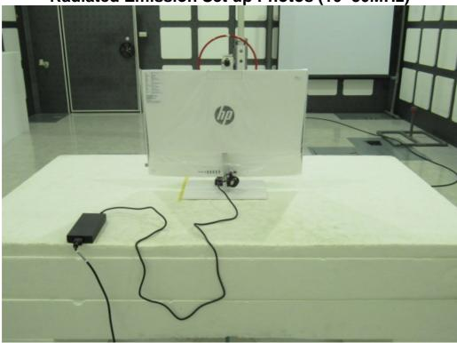
Radiated Emission Set up Photos (30MHz~1GHz)
