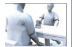
In this configuration, the Recorder is up on the kickstand. The subject is in view of the back camera and the interviewer is in view of the front camera.
