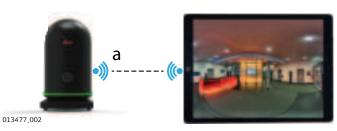
a Raw data transfer from BLK360 to computing device. Refer to Connecting to a computing device using Wi-Fi step-by-step.
