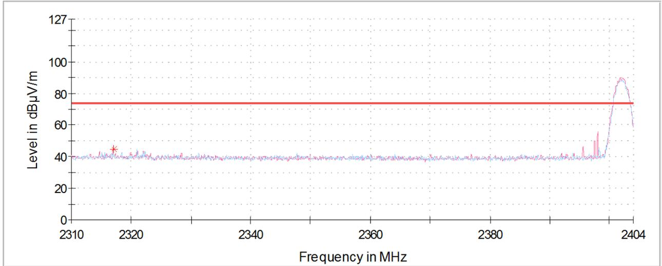
**- 8DPSK \_ Highest channel (2 480 MHz)\_ Module 1**
