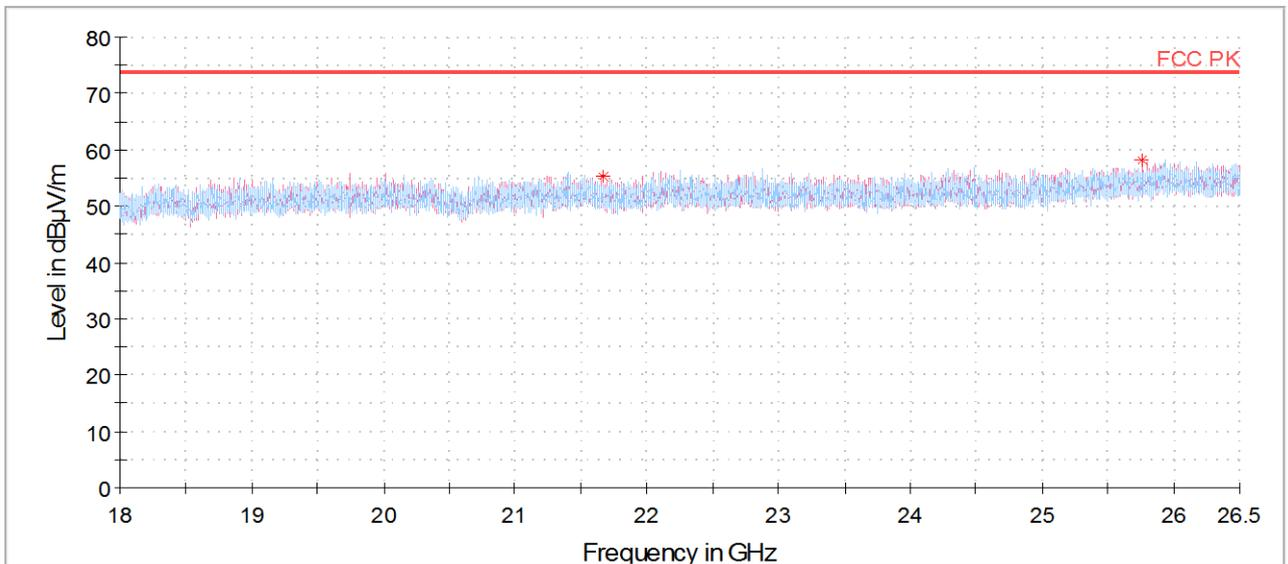
Figure 8. Restricted Bandedge data (Radiated)
