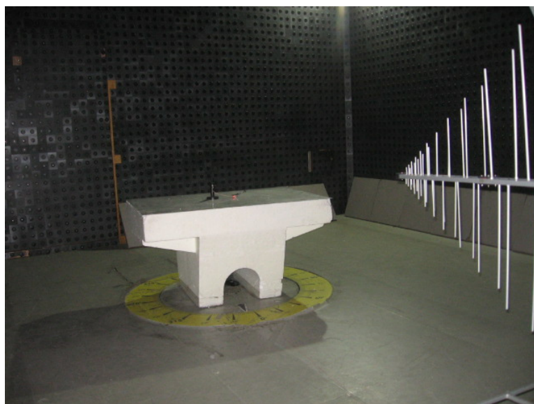
Photograph 8.2.1 Setup for preliminary radiated emission measurements
