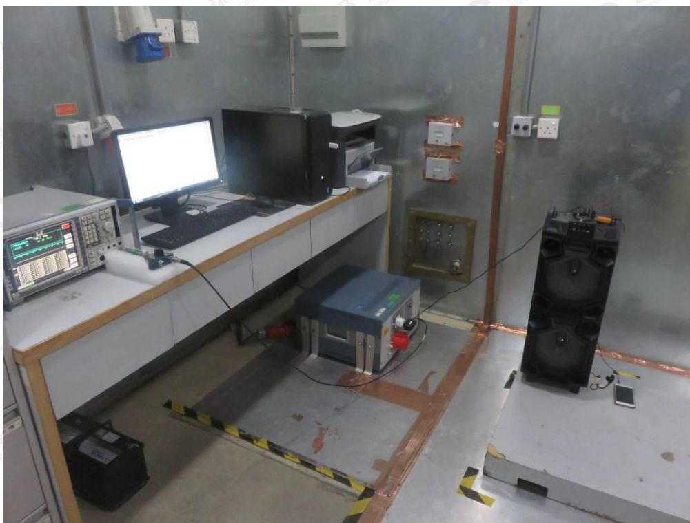
FCC RADIATED EMISSION TEST SETUP
