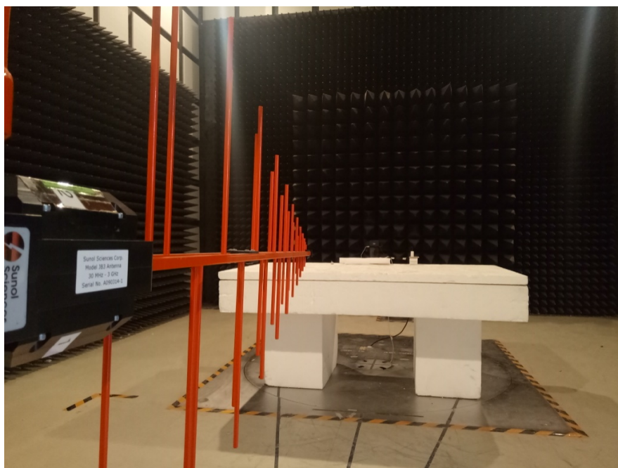
Radiated Emissions View (1GHz-18GHz)
