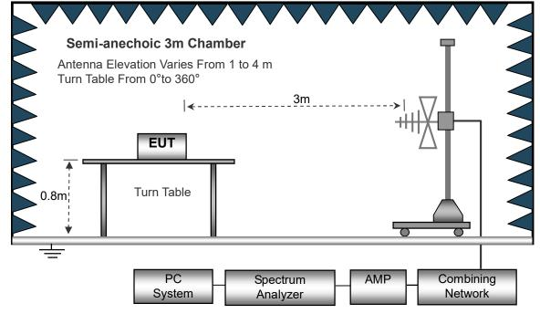
(C) Radiated Emission Test-Up Frequency Above 1GHz
