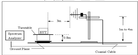
(C) Radiated Emission Test-Up Frequency Above 1GHz
