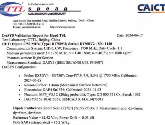
SAR(1 g) = 9.09 W/kg; SAR(10 g) = 4.88 W/kg Smallest distance from peaks to all points 3 dB below = 9.5 mm Ratio of SAR at M2 to SAR at M1 = 56.8% Maximum value of SAR (measured) = 13.8 W/kg
