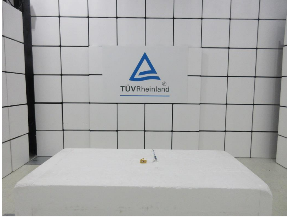
Photograph 2: Test Setup for Spurious Emissions (Front View 2)
