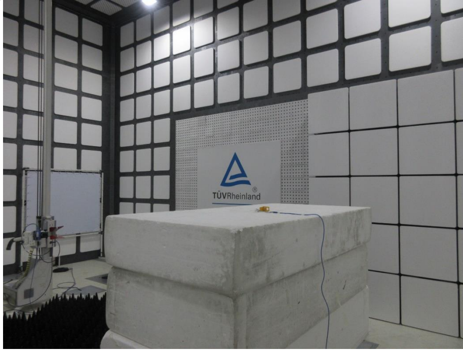
Photograph 6: Test Setup for Spurious Emissions (Back View 4)
