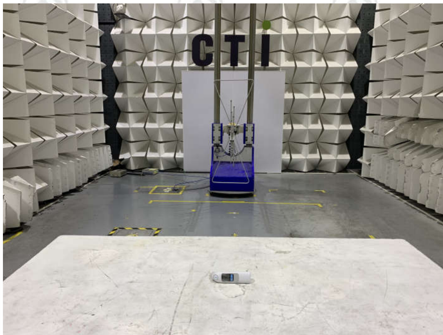
Radiated spurious emission Test Setup-1(Below 1GHz)
