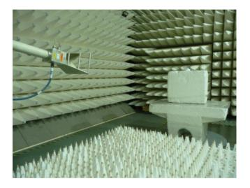
Photograph No.5 Setup for 20 dB bandwidth measurements
