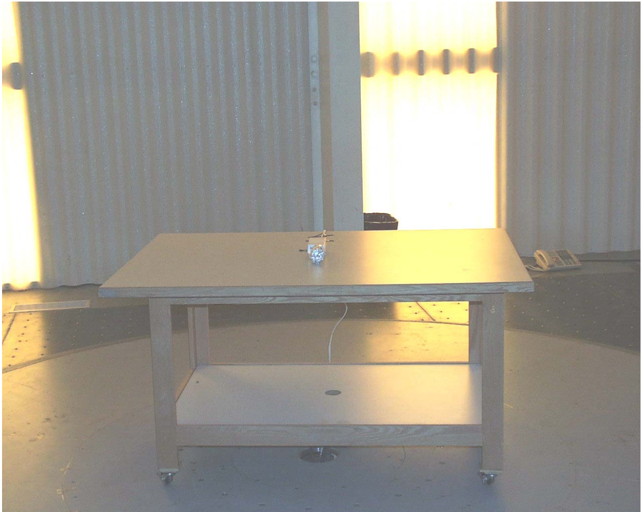
Photograph 1 - Front View Radiated Disturbance Worst Case Configuration
