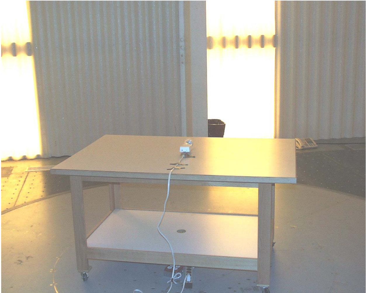
Photograph 2 - Back View Radiated Disturbance Worst Case Configuration
