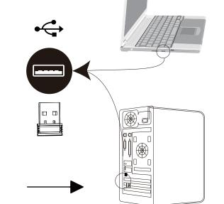
Press the FN+1 key combination ON the keyboard to switch to 2.4G mode, and dial the two-gear power switch to the state of "ON". At this time, the receiver can be inserted in a close distance and used normally.
