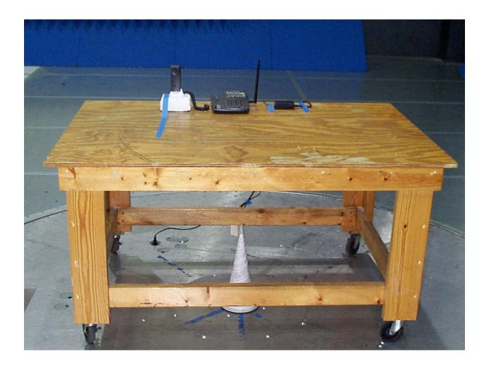
Figure 11-1: Configuration photograph, radiated emission, front view
