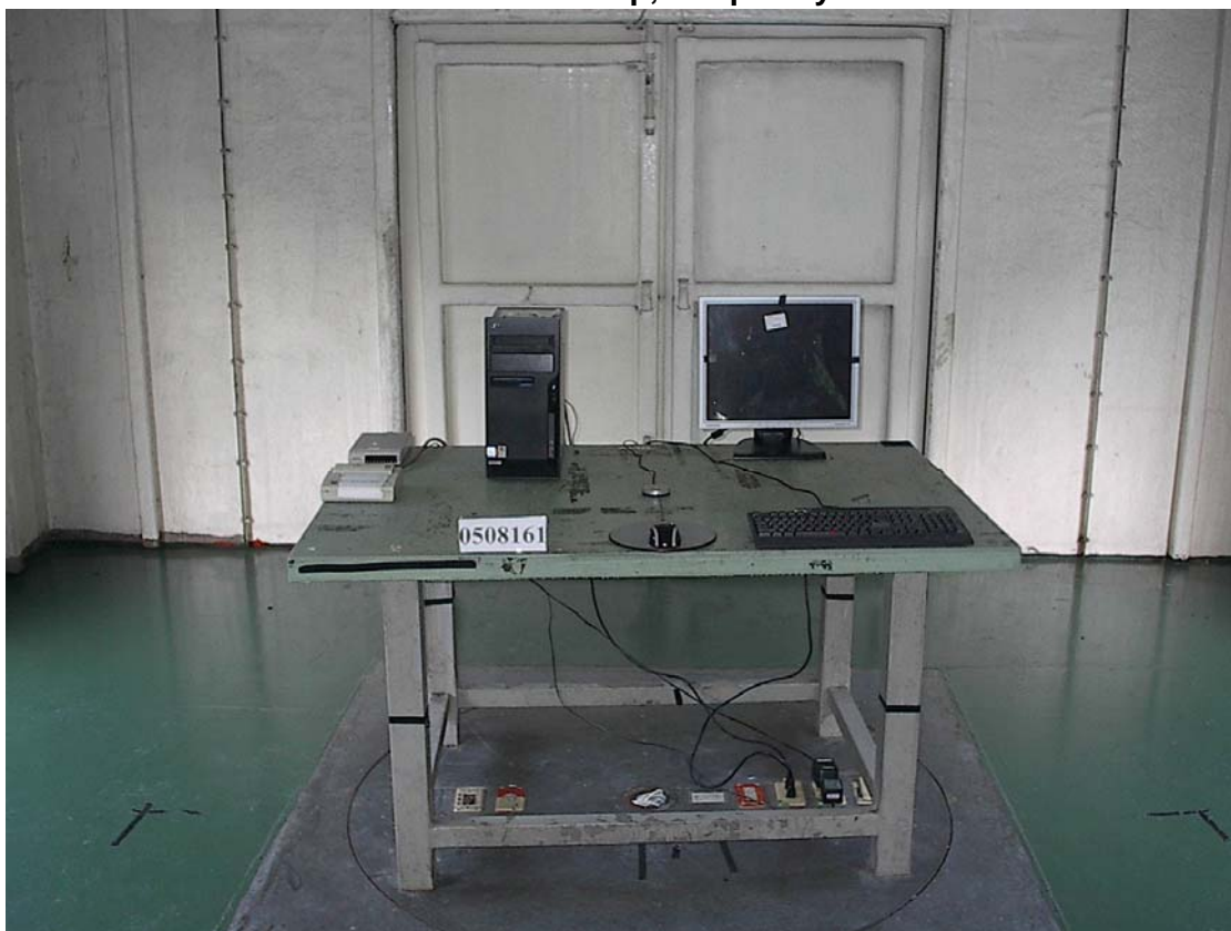
Radiated Emission Test Set-up, Frequency Below 30MHz
