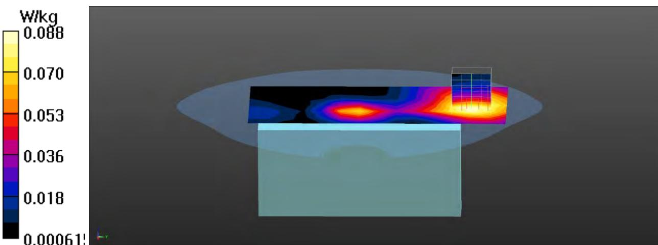
**WCDMA RMC Band 4 EUT Bottom (Body-10mm) Z-Axis plot
