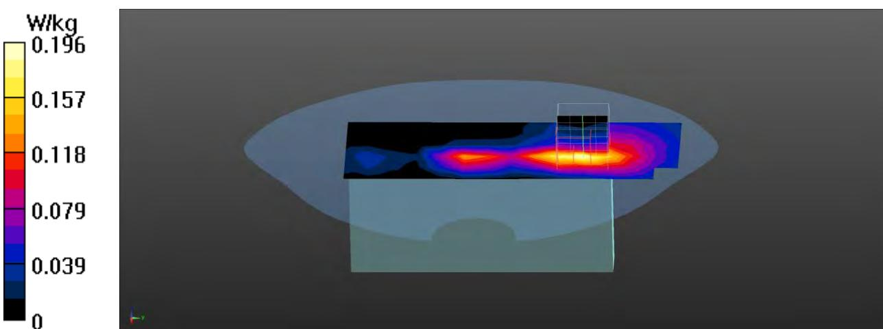
**LTE Band 4 QPSK 20M 1RB EUT Bottom (Limb-0mm) Z-Axis plot**
