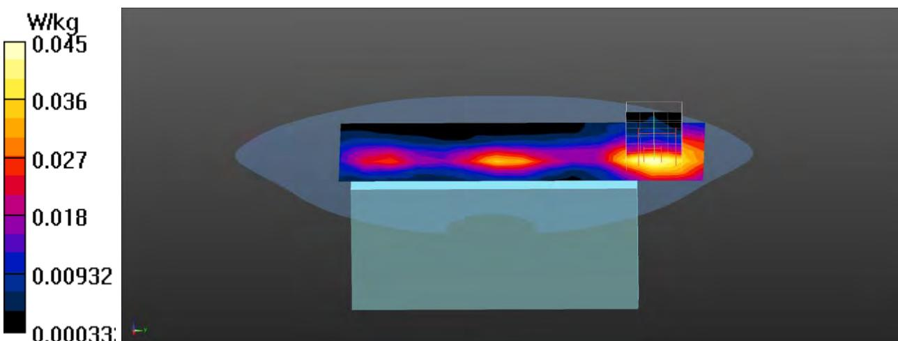
**PCS 1900 GPRS 4UP EUT Back (Body-10mm), Z-Axis plot**
