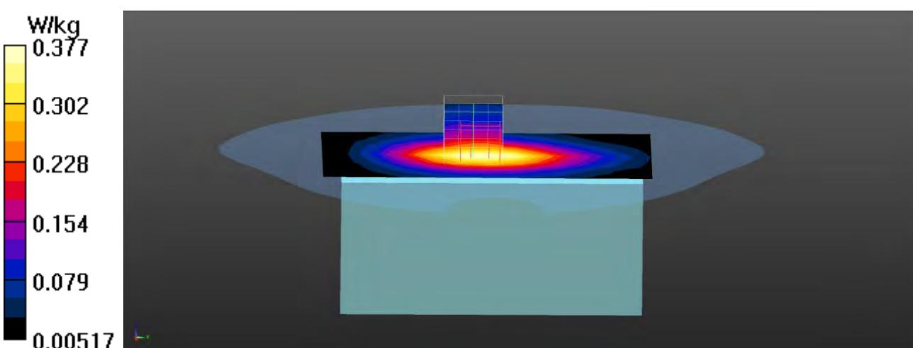
**GSM 850 GPRS 1UP EUT Back (Body-10mm), Z-Axis plot
