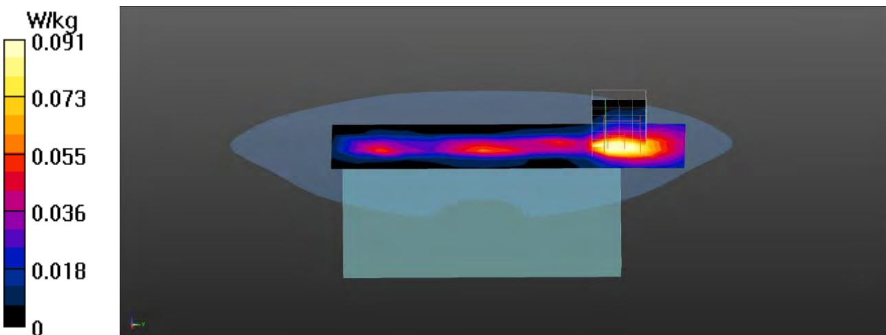
**WCDMA RMC Band 2 EUT Back (Limb-0mm) Z-Axis plot
