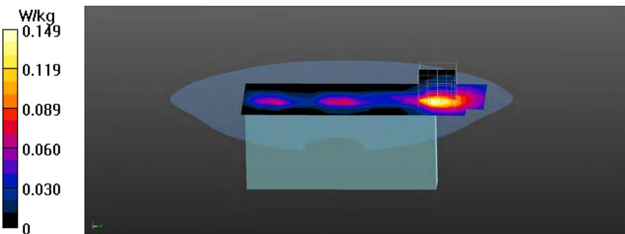
**LTE Band 2 QPSK 20M 1RB EUT Back (Limb-0mm) Z-Axis plot**
