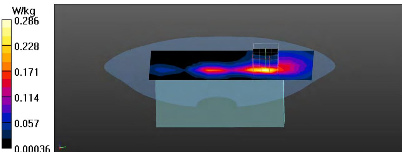
**WCDMA RMC Band 4 EUT Bottom (Limb-0mm) Z-Axis plot
