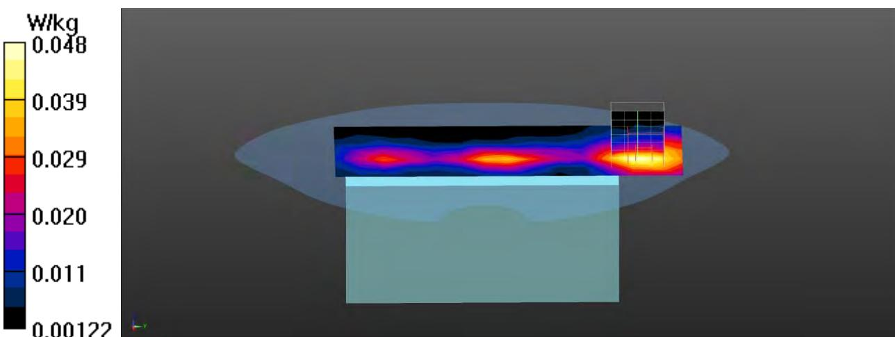
**WCDMA RMC Band 2 EUT Back (Body-10mm) Z-Axis plot
