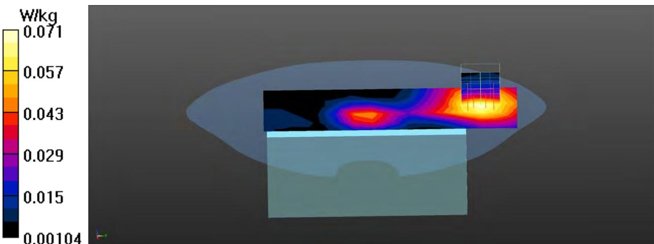
**LTE Band 4 QPSK 20M 1RB EUT Bottom (Body-10mm) Z-Axis plot**
