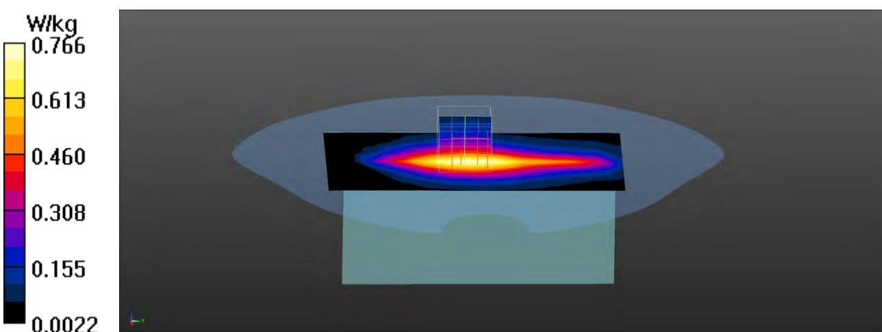
**GSM 850 GPRS 1UP EUT Back (Limb-0mm), Z-Axis plot
