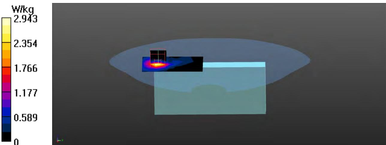
**802.11a EUT Top (Limb-0mm), Z-Axis plot
