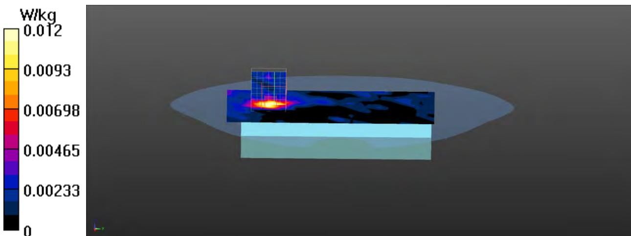
**802.11b EUT Front (Body-10mm) Z-Axis plot
