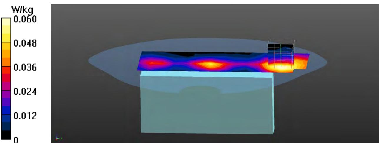
**LTE Band 2 QPSK 20M 1RB EUT Bottom (Body-10mm) Z-Axis plot
