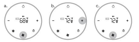
When turning on CozyPod, it will display the room temperature. Eco Mode means that the CozyPod will automatically turn off when the desired room temperature is reached. When the temperature falls two degrees below the set temperature, the CozyPod will turn back on until the desired temperature is reached.
