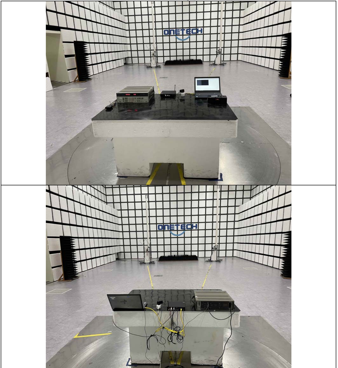
Radiated Emission Test Set Up (Below 1 GHz)
