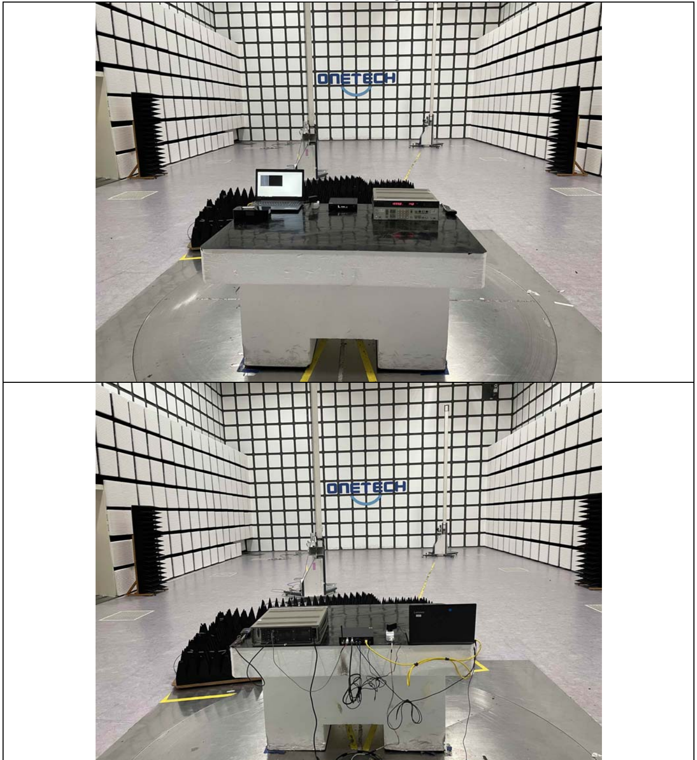
Radiated Disturbance Test Set Up (Above 1 GHz)
