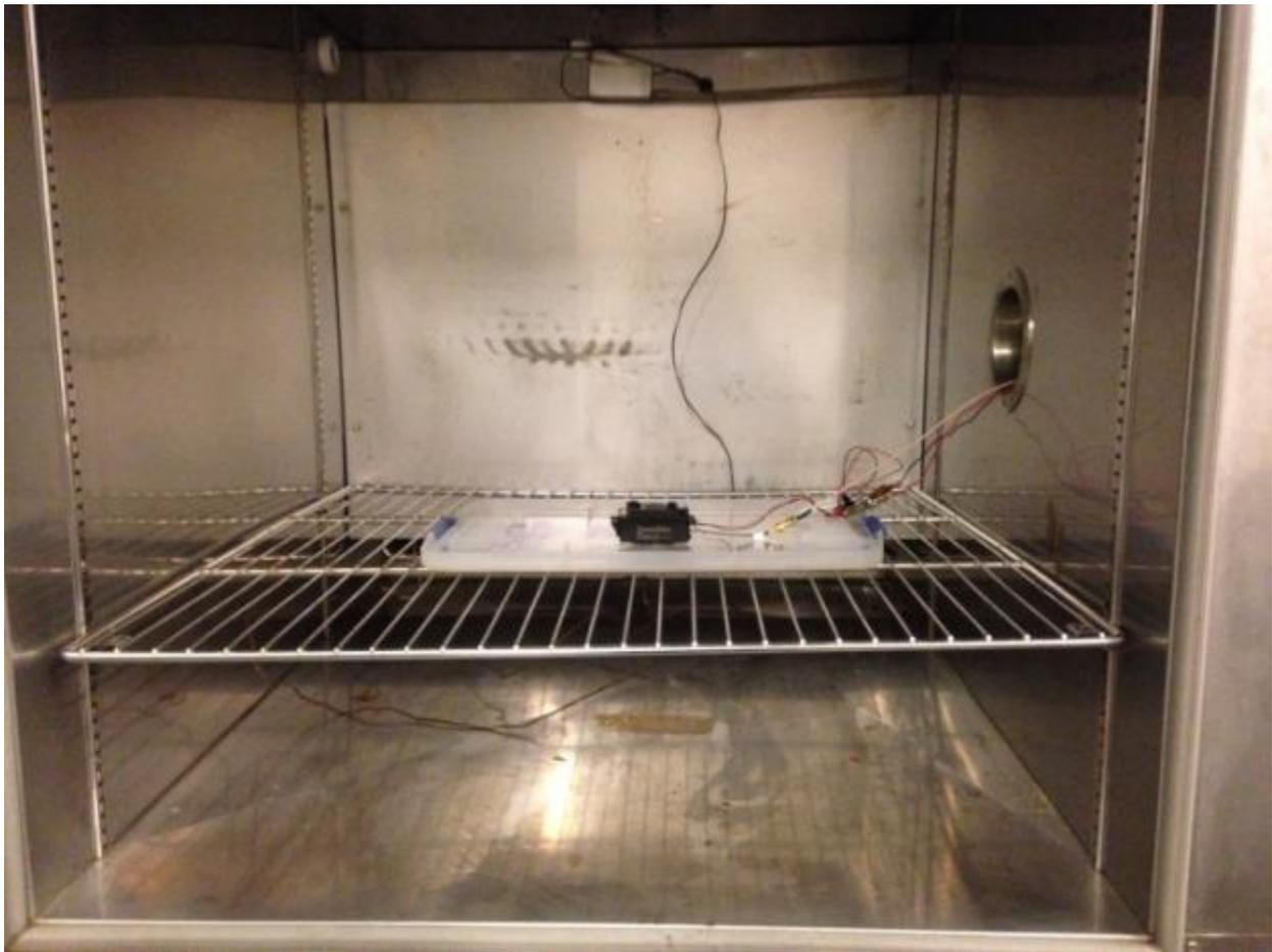
**Figure 6. Frequency Stability Test Setup**
