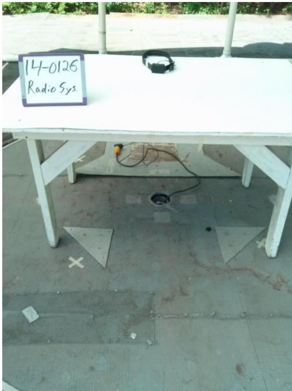
**Figure 1. Radiated Emissions Test Setup (Front)**
