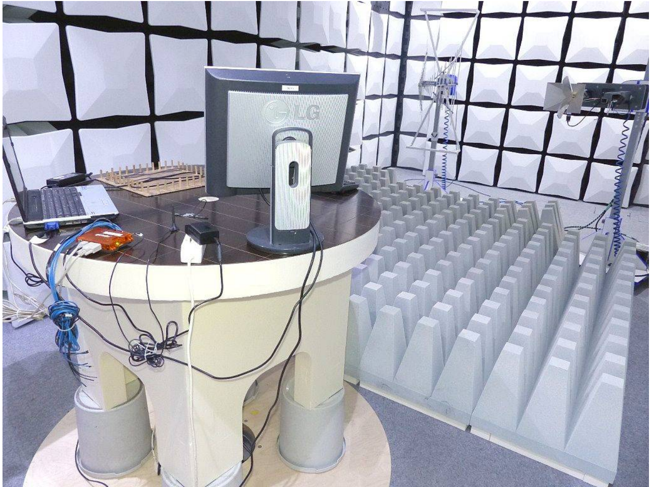
Photo 2: Test setup for radiated measurements (Enclosure, fully-anechoic chamber, 1-3 GHz, unintentional radiator §15.109, ANSI C63.4)
