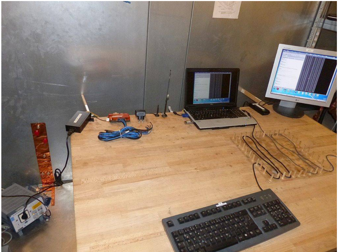
Photo 5: Test setup for conducted measurements (computer peripheral setup, EUT supplied by PoE injector, measured at power-over-Ethernet injector, unintentional radiator §15.107, ANSI C63.4)
