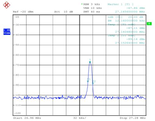
The results: The unit does meet the FCC Part 15 C Section 15.227 requirements.
