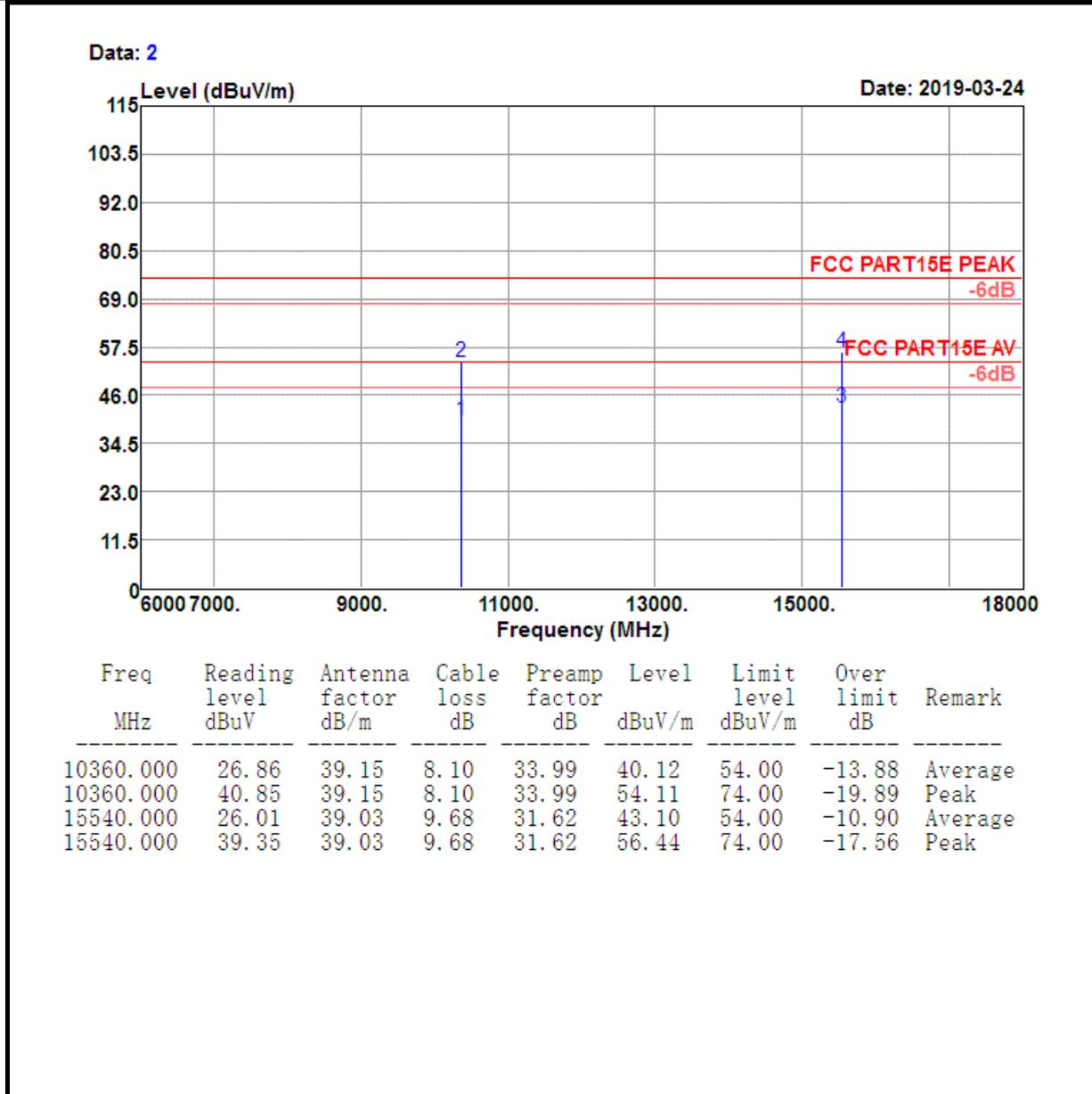
Note: Emission was scanned up to 40GHz; No emissions were detected above the noise floor which was at least 20dB below the specification limit.
