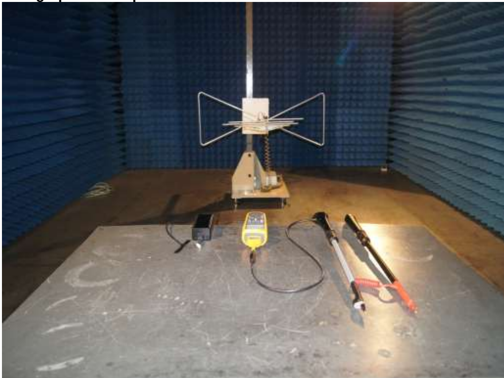
Photograph 2: Set-up for Radiated Emission – 30-1000 MHz
