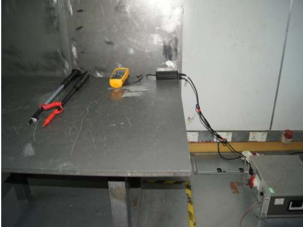
Photograph 1: Set-up for Conducted Emission
