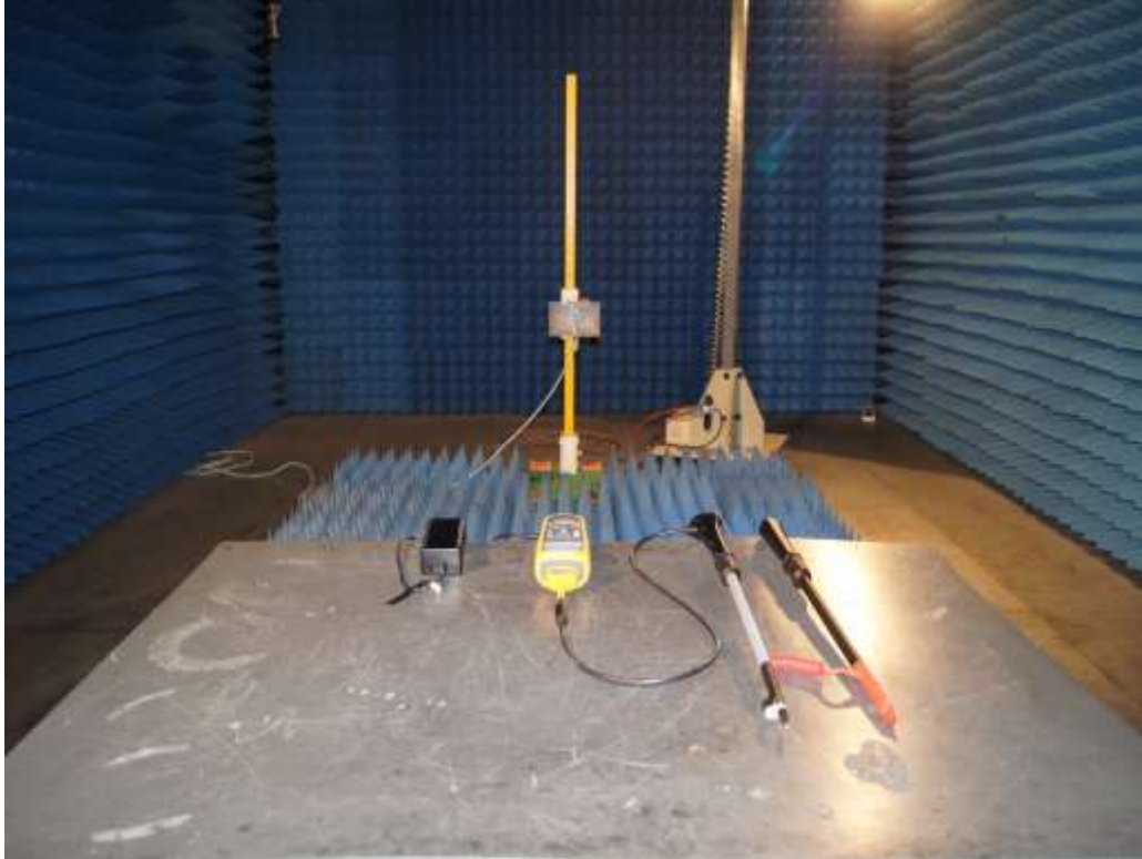
Photograph 3: Set-up for Radiated Emission – 1-18 GHz
