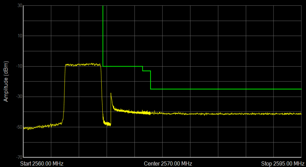
Band7 QAM16 BW=5MHz Channel=21425 RB Size=25 Position=#0
